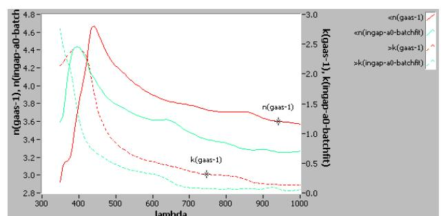
Fig.4: Dispersion functions  $n$  and  $k$  of GaAs laser bulk and InGaP anti-reflection coating obtained from batchprocessing of Delta/Psi spectra of laser A ROI 0, wavelength lambda in nm
