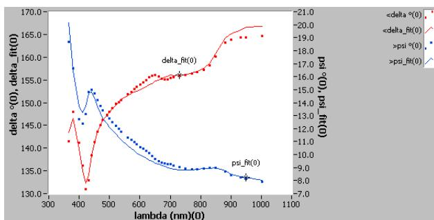
Fig.3: Spectra of Delta/Psi of InGaP coating in ROI 0 on laser D. Fit with the following model parameters: VIS-oscillator: frequency  $1.74 \pm 0.02$ , amplitude  $-0.42 \pm 0.07$ , damping  $0.28 \pm 0.06$ , UV-oscillator: frequency  $28000 \pm 6000 \text{ cm}^{-1}$ , amplitude  $3.8 \times 10^9$ , damping  $6200 \pm 4000$ , background: refractive index  $n = 2.457 \pm 0.008$  and extinction  $k = 0$ , thickness  $9.97 \pm 0.15$ , mean square error 10.5
