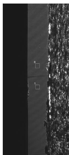
Fig.2: Ellipsometric contrast image ( $0.4 \text{ mm} \times 0.8 \text{ mm}$ ) of the front facet of a laser,  $70^\circ$  angle of incidence, 532 nm wavelength
