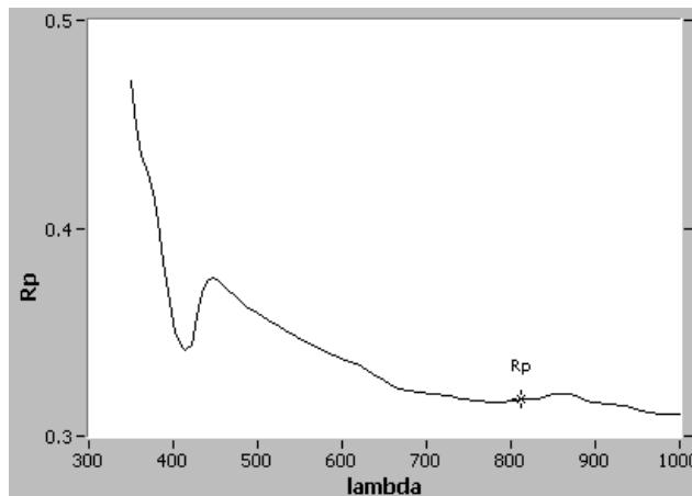
Fig.5: Optical field-reflectivity  $R_p$  of the InGaP coated GaAs laser vs. wavelength close to 0° angle of incidence
