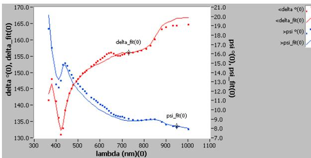
Fig.3: Spectra of Delta/Psi of InGaP coating in ROI 0 on laser D. Fit with the following model parameters: VIS-oscillator: frequency  $1.74 \pm 0.02$ , amplitude  $-0.42 \pm 0.07$ , damping  $0.28 \pm 0.06$ , UV-oscillator: frequency  $28000 \pm 6000 \text{ cm}^{-1}$ , amplitude  $3.8 \cdot 10^9$ , damping  $6200 \pm 4000$ , background: refractive index  $n = 2.457 \pm 0.008$  and extinction  $k = 0$ , thickness  $9.97 \pm 0.15$ , mean square error 10.5
