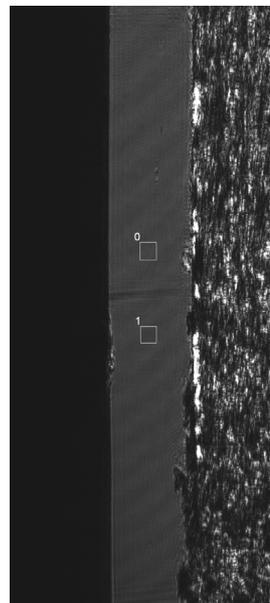
Fig.2: Ellipsometric contrast image (0.4 mm x 0.8 mm) of the front facet of a laser,  $70^\circ$  angle of incidence, 532 nm wavelength
