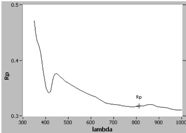
Fig.5: Optical field-reflectivity  $R_p$  of the InGaP coated GaAs laser vs. wavelength close to  $0^\circ$  angle of incidence
