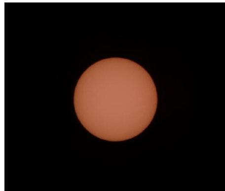
Figure 2. A photograph of the sun, taken through suitable neutral density filters, can be integrated and calibrated against a measured direct normal irradiance value. With that process, a standard camera then provides a quantitative measure of energy per sensor pixel-value increment.
