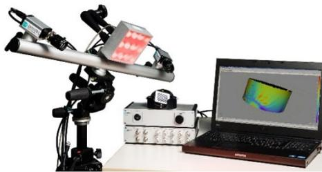
Figure 11 - DIC System with two cameras and illumination option
