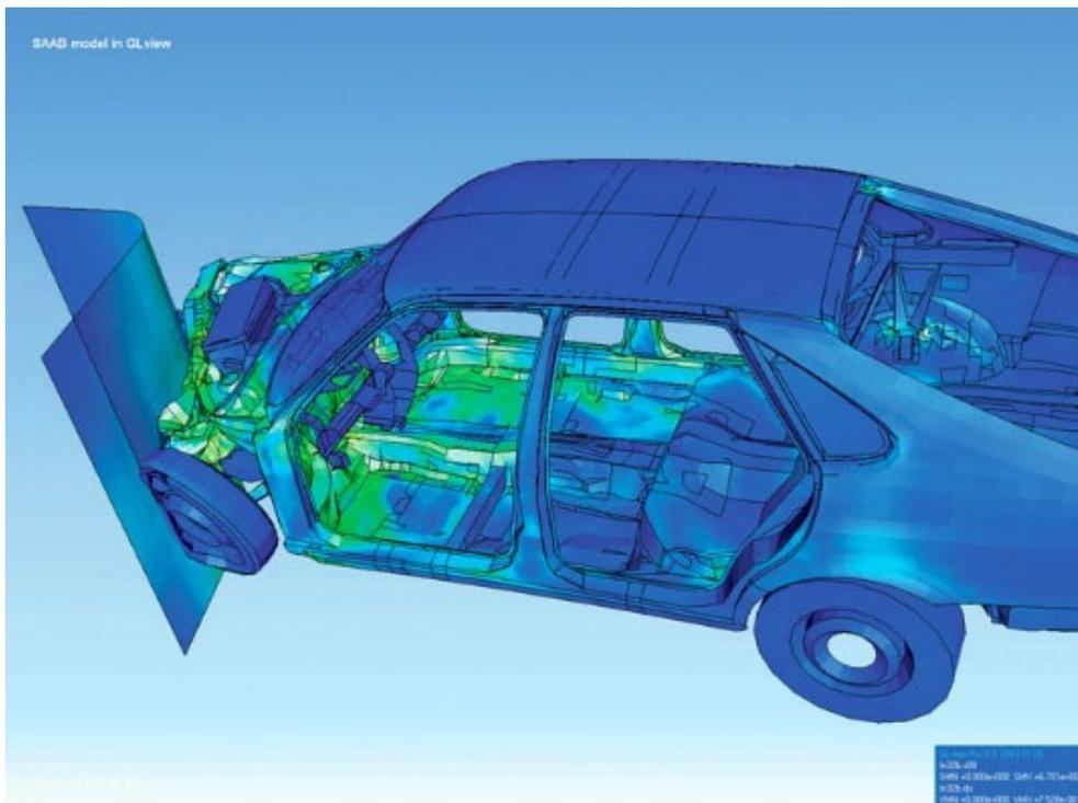
Figure 1 - Visualization of how a car deforms in an asymmetrical crash using finite element analysis
