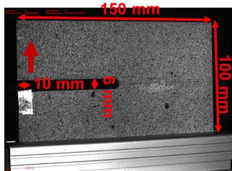
Figure 3 - Compact Tension Sample
