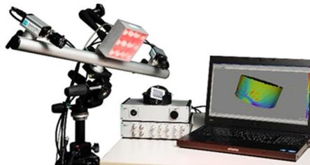
Image 6: Q-400 DIC System with two cameras and illumination option
