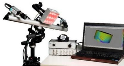
*Q-400 Digital Image Correlation System with two cameras and illumination option*
