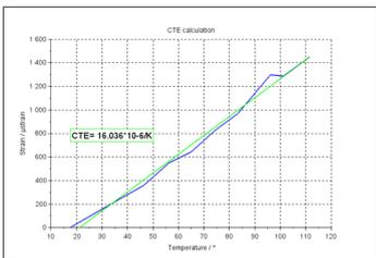
*Thermal expansion coefficient (CTE) calculation*
