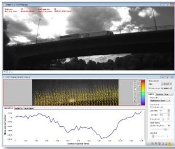
*Bridge displacement under load of passing truck*
