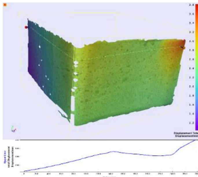
Figure 5 - Deformation of a cardboard box
