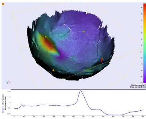
Figure 13 - Displacement of hemisphere object
