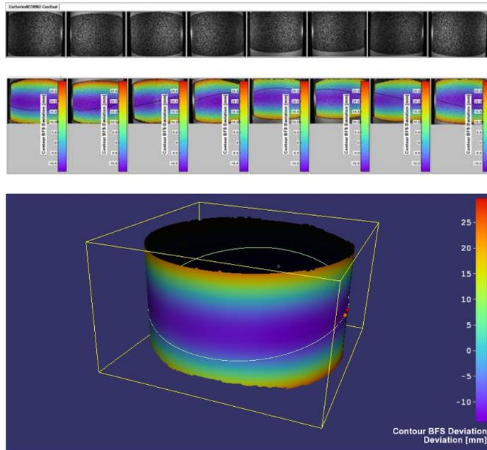
Figure 2 - Full-field evaluation of a cylindrical object with an 8 camera DIC System
