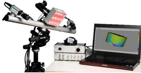
Figure 14 - DIC System with two cameras and illumination option
