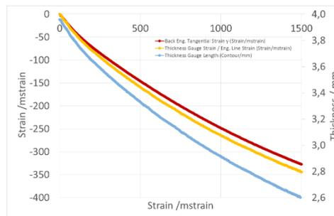
Figure 9 - Thickness changes, strain in thickness and perpendicular to direction of the load
