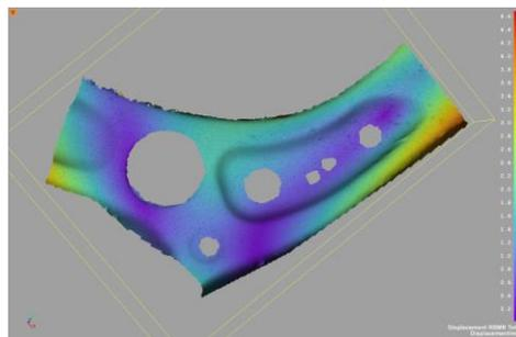
Figure 10 - Two camera DIC measurement limited to surface only, not showing shadowed areas.
