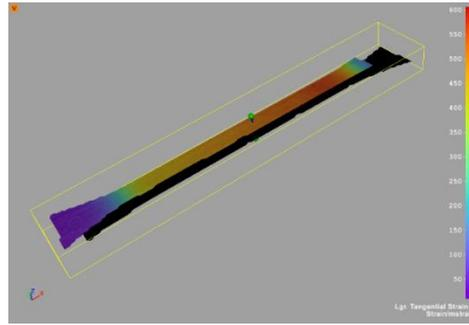
Figure 7 - Front and backside strain in loading direction tensile test sample as 3D model
