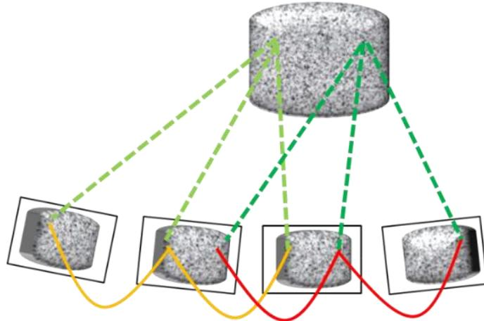
Figure 4 - Definition of facets in a multi camera DIC setup using the cluster approach
