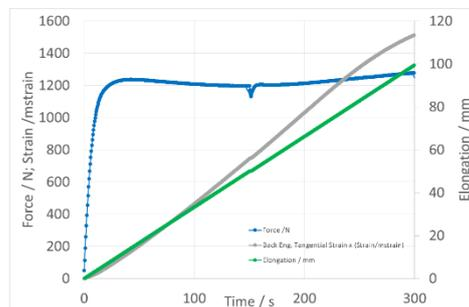
Figure 8 - Traverse displacement, force and strain in loading direction over time
