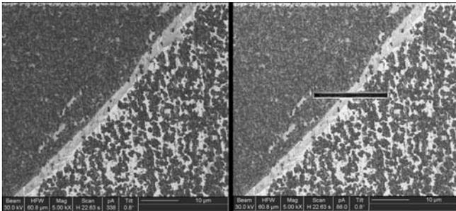
Figure 2: Before and After slotting FIB images
