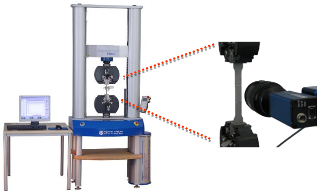
RTSS set up on a tensile test machine
