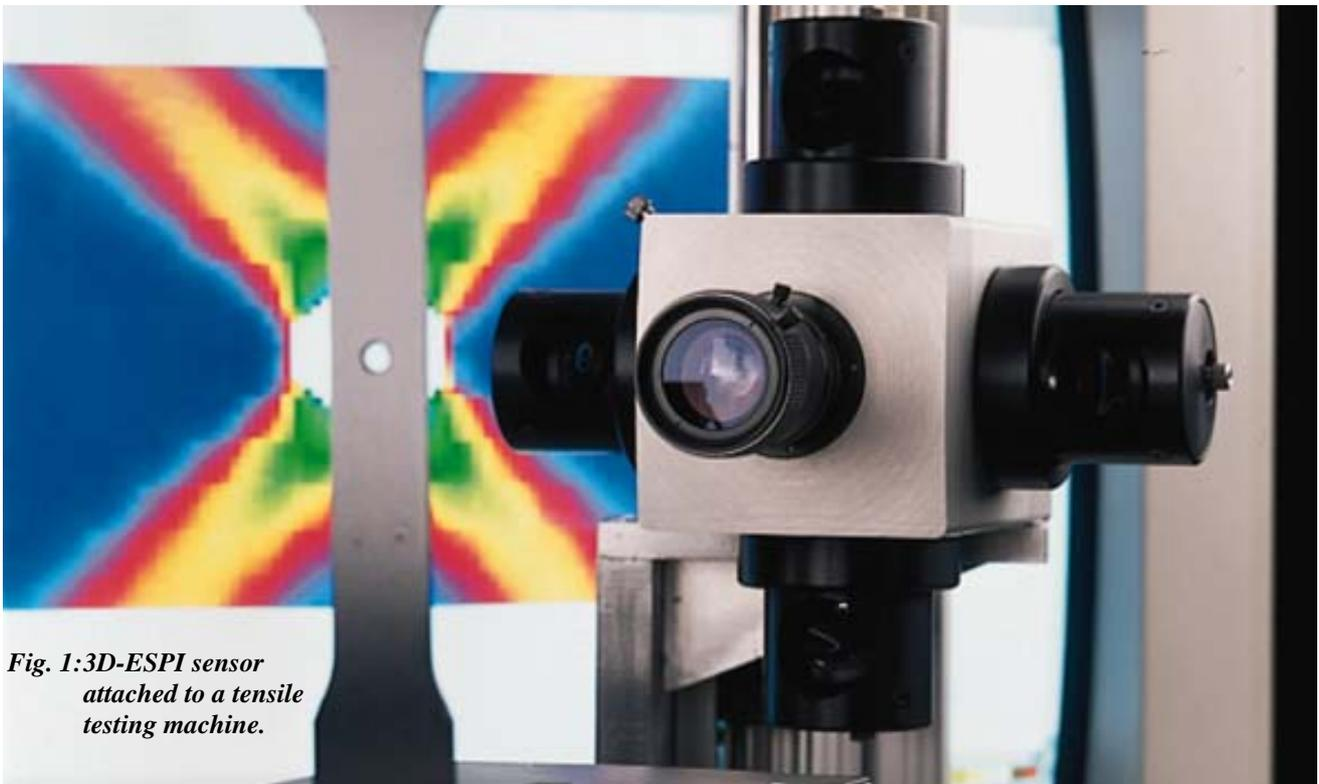
*Fig. 1: 3D-ESPI sensor attached to a tensile testing machine.*
