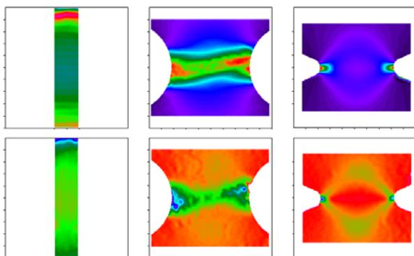
*Fig. 3: Strain distribution of three different samples of titanium. Upper row is the longitudinal strain field, the lower is the transverse strain field.*
