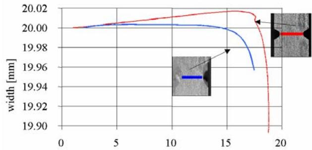
*Fig. 7: In-plane movement of the notched specimen at elastic (left) and plastic (right) behavior.*
