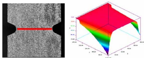
*Fig. 5: Variation of the transverse strain as a function of the position across the notch and the measurement steps. The red line indicates the line where the values for the diagram have been taken.*
