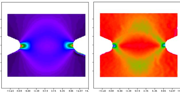
*Fig 2: Strain distribution of a notched titanium sample, load 18000N, thickness of 1.5 mm, width in notch ground 20 mm. Left: longitudinal strain field, right: transverse strain field*
