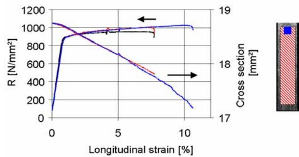
*Fig 4: True stress-/true strain diagram for the parallel sample. The shorter curves are the average values over the sample.*
