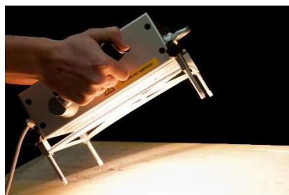
Figure 5 - Various tungsten heaters, from 375W to 3000W
