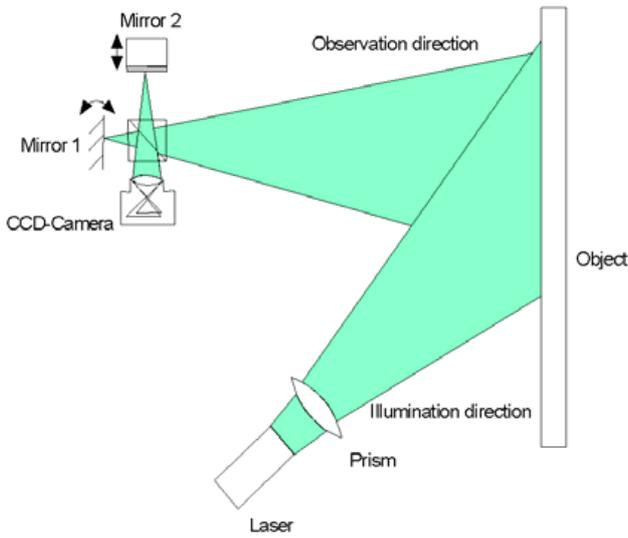
Fig.2: Schematic diagram of a shearography system.
