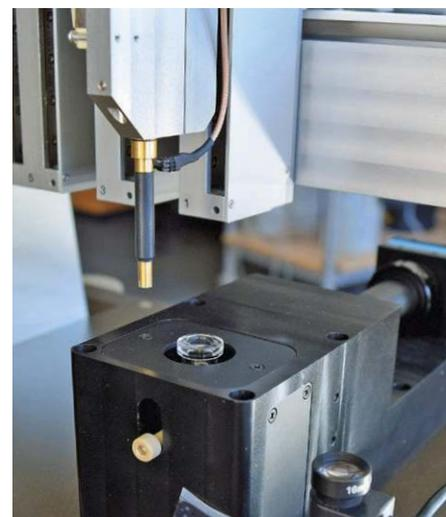
Micro-powder dispenser above a piezo-actuated powder reservoir. Two control cameras inspect the loading from the side and from below. Depending on the tip structure, different amounts of beads can be transferred.
