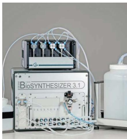
The F-Box, the electronic brain of the instrument and also central control station for pressure, vacuum and liquids, plus bottles with liquid level control and four syringe pumps for dispensers
