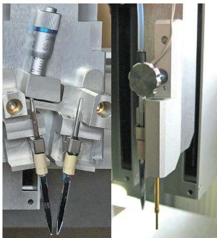
Twin tip pipetting device (left), swivelled. Teflon tubes to piezo dispensers are missing. On the right, an (old) Z-sensor, side by side with a single piezo tip.
