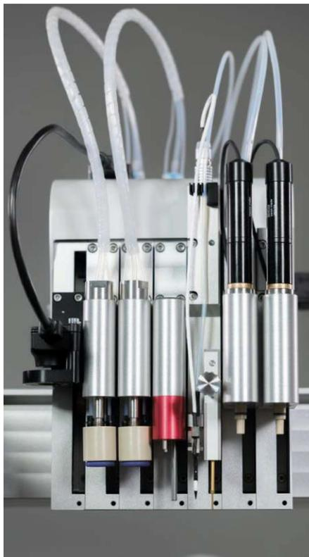
Example of a fully equipped pipetting head with (1) camera, (2+3) gripper/3-lumen pipette (one tool!), (4) FlipTube opener, (5) piezo tip + Z-sensor on one Z-axis, (6+7) nozzles for single-use needles and tips
