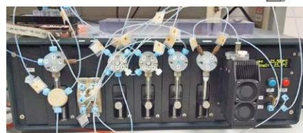
Detail of the GeSiM Fluidics software (example) and corresponding F-Box with selector valves, syringe pumps and Peltier cooler with temperature control
