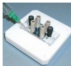
Injection of PDMS into the casting station. The silicon master lies under the transparent lid. Please note the channel spacers (brown fittings).
