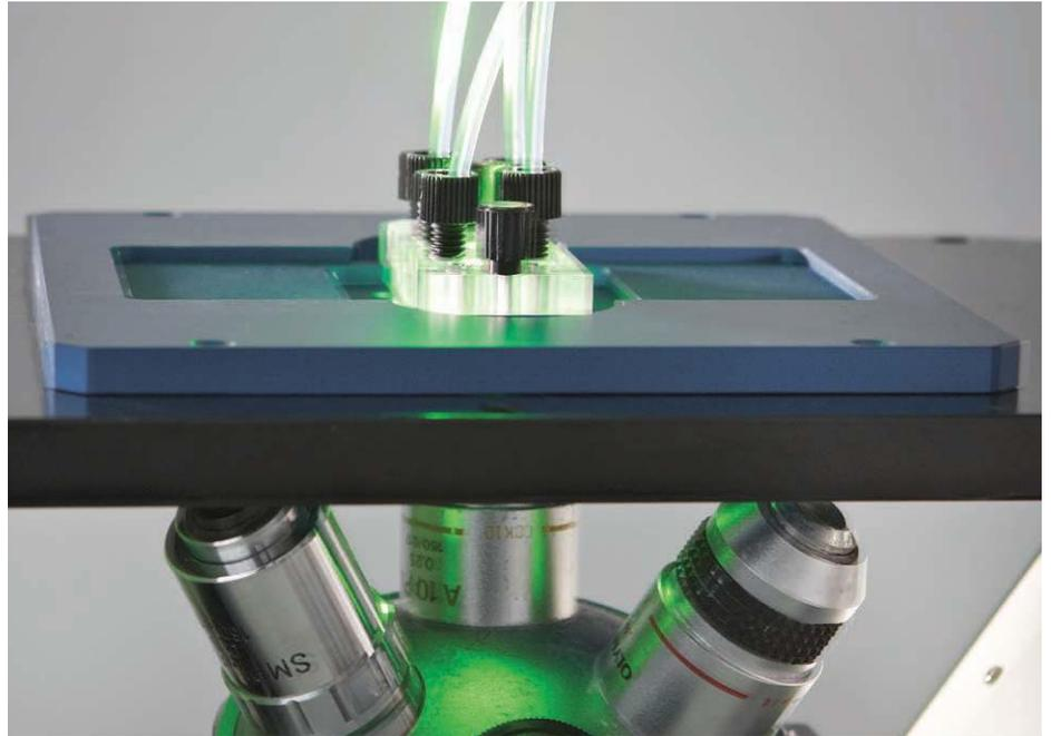
The MicCell is set up by casting a polymer channel plate, adding a coverslip, mounting it in the support and doing experiments under microscope control. The MicCell is ideal for rapid prototyping; making a new channel requires only a new silicon master that you can order from GeSiM.
