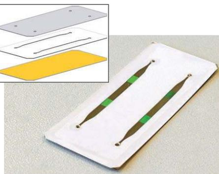
Biosensor cell made of three foils: transparent cover foil with holes, white channel foil, PC foil with four sensor pads (nanoimprinted in a GeSiM  $\mu$ CP4.1 and gold-coated). Used in a MicCell with near-infrared LEDs and wavelength-dependent photodiodes.
