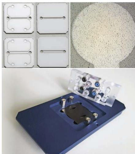
Foil chips for gradients made of four foils (22x22, front/rear view), pore membrane (top right) and PC body with O-rings on the MicCell support (bottom)
