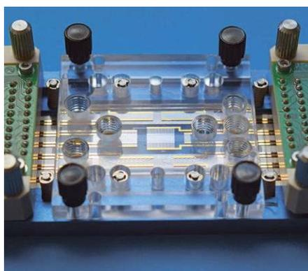
MicCell with microelectrodes structured on a 25x75 coverslip and connected via spring-loaded contacts
