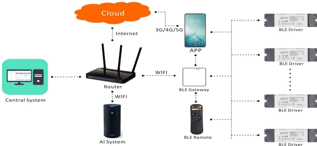
BLE Sigmesh Smart Lighting System
