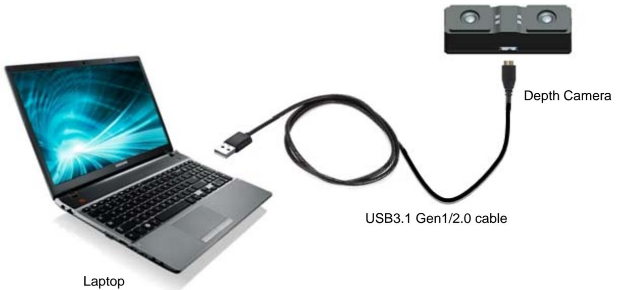
**Figure 3-1. Depth Camera to PC Connection**
